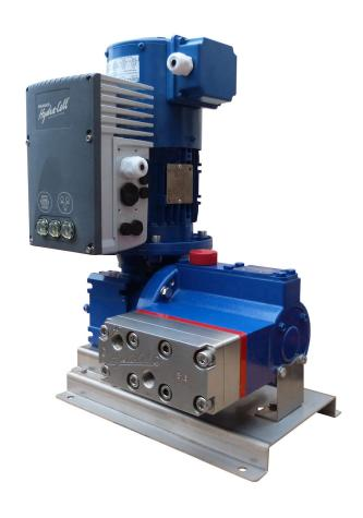
Built with Aflas diaphragms, PTFE fluid-end o-rings and FKM drive case o-rings, the first P200 pump performed exceptionally well, eliminating the low-efficiency, high-shear, and non-lubricating pumping problems. The outcome was so successful that Hydra-Cell P200 pumps have been steadily replacing the gear pumps on the customer's systems installed in automotive plants around the world.
