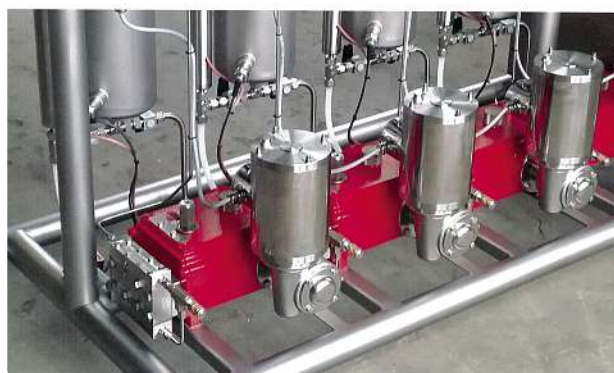
Battery of Hydra-Cell MT8 metering pumps on extrusion system at pet food plant.
