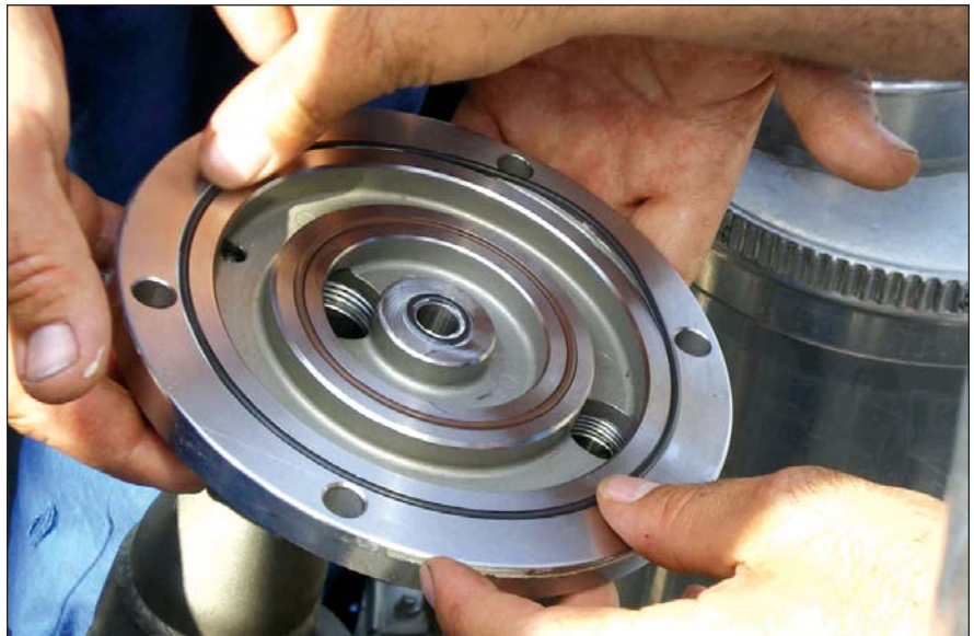
Simple build, low maintenance. This Hydra-Cell pump manifold inspected by Romgaz engineers after 1800 hours continuous operation showed no signs of wear.
