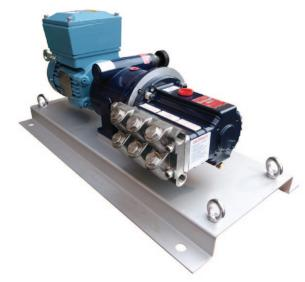
Wanner International has introduced two new Hydra-Cell® Dosing Performance Pump ranges with mechanical flow rate adjustment. Because seal-less Hydra-Cell pumps are true positive displacement pumps, flow rate is directly proportionate to input shaft speed and virtually independent of system discharge pressures. Very precise, infinite adjustment of shaft speed is achieved through a simple manual adjust hand wheel.
