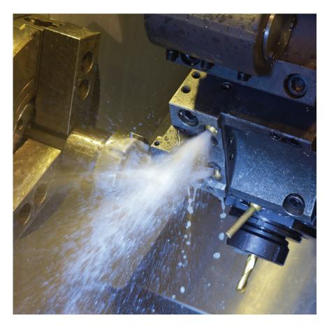
High Pressure Coolant Delivery is extremely popular in aerospace manufacturing in order to machine lightweight, advanced engineering alloys more effectively and economically.
