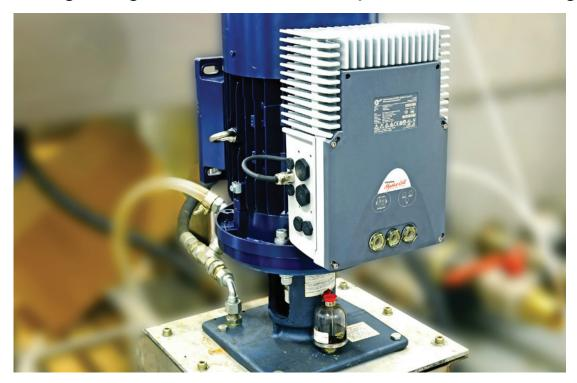
Wanner International has introduced the Hydra-Cell Intelligent High Pressure Coolant Pump that it claims can save machine tool operators up to 70% of their pump energy costs.
