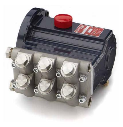
A further benefit of the Hydra-Cell with Mono-Block pump head is its ability to prime quickly at slow speeds. Mono-Block pump heads are available in brass or 316 stainless steel. Diaphragms are available in a range of materials from PTFE and Viton to Buna, Neoprene and EPDM, to suit the requirements of the liquid being pumped.
