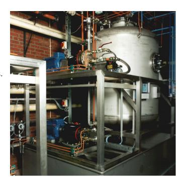
Compact and with a small footprint, Hydra-Cell® pumps are also designed to run-dry without incurring damage; further system protection should the feedstock run out and a guard against operator error. They can pump feed materials with a wide viscosity range and can also handle corrosive liquids.
