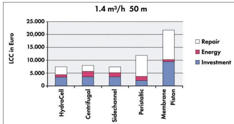
Figure 2a: LCCs for Pumps Delivering 1.4 m<sup>3</sup>/hr at 5 bar. (F-W Hennecke)
