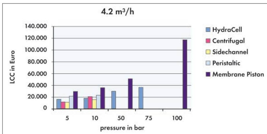
Figure 2b: LCCs for Pumps Delivering 4.2 m³/hr at Various Pressures. (F-W Hennecke)
